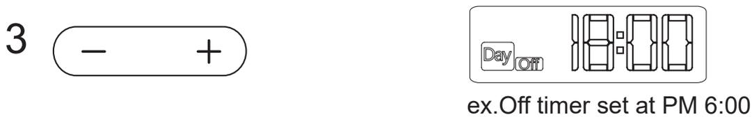
Press the button “ + ” or “ - ” to set the time. After the time is set, the timer will start or stop automatically.
