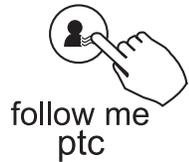
Press the Follow me/PTC button for 2 seconds or more to activate the PTC function, when the unit is under the Heat mode.
